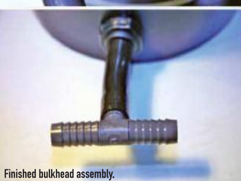
Cut 3/4" vinyl for T assembly and connection.
